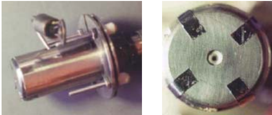
Figure 2.3 Cathode and keeper assembly with close-up front view of the keeper and cathode orifices.
