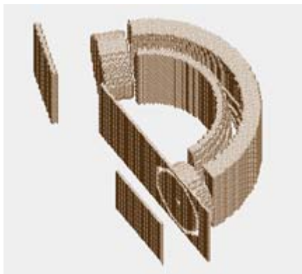
Figure 8.5a The ESA geometry in SIMION 3D 7.0. Electrode potentials are applied to simulate the electric fields seen by the ions.
